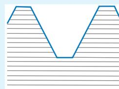
Fibre course of a cut internal thread
