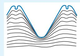
Fibre course of a rolled internal thread
